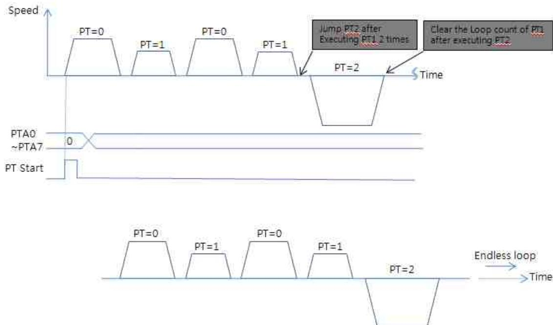
\* Refer to the sample file for testing Position Table, 'PTsample (Loop counter clear).fpt'.
