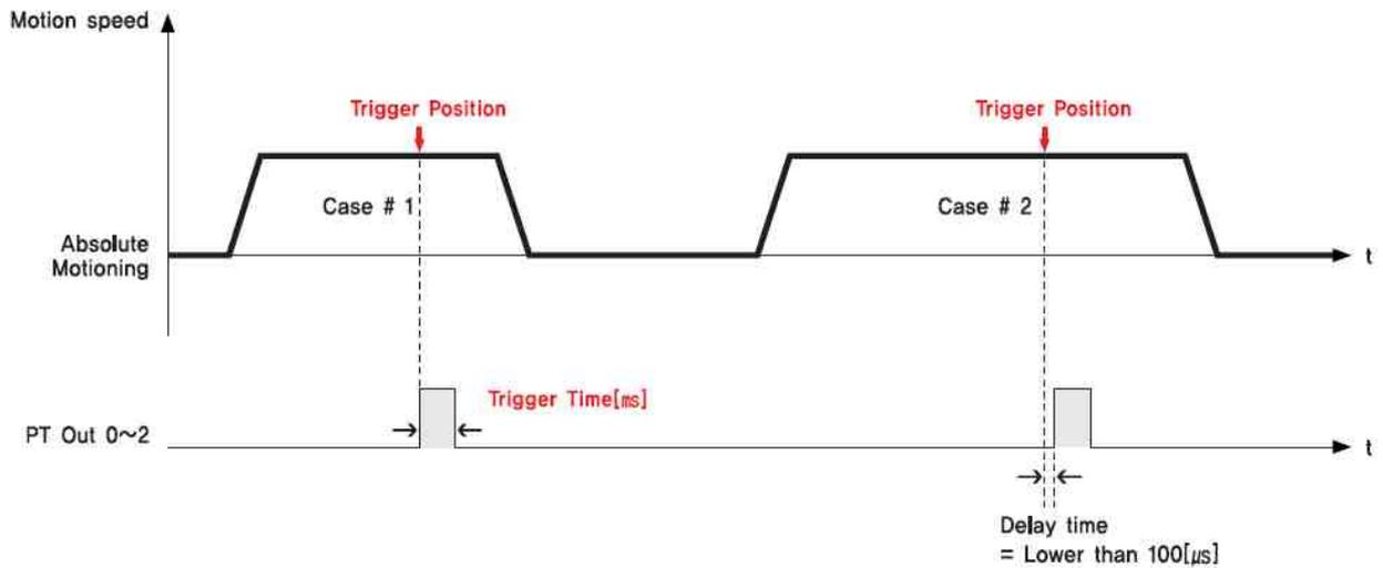
\* The signal pulse width of PT Output is set by 'Trigger Time' value.
