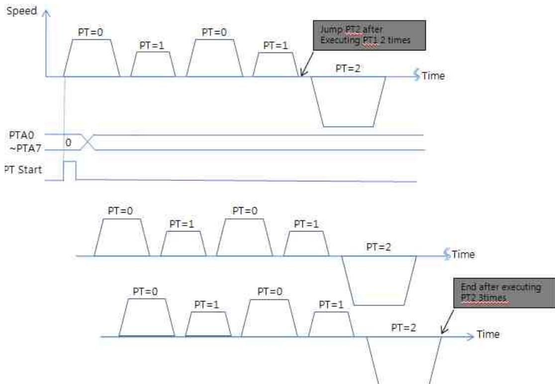
\* Refer to the sample file for test ing Position Table, 'PTsample (Loop Motioning) .fpt
